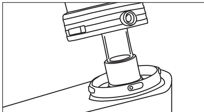
4. Lift the UV light tube cover up to remove it and expose the Quartz Sleeve.
