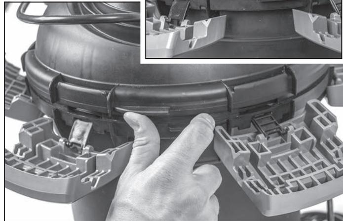
2. Once the clips are released, use the lid and tank tabs to gently lift the lid assembly free from the canister. The lid may be difficult to lift due to the pressure inside the filter. Loosening one of the plumbing fittings will reduce the pressure, making it easier to remove the lid.
