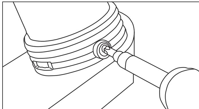
3. Remove the set screw holding the UV light tube in place under the UV Ballast. Please note: use a properly-sized Phillips screw driver small enough to grip the set screw.
