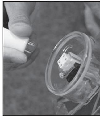
6. Grip the base of the UV bulb and pull it free from the four-pronged socket.
