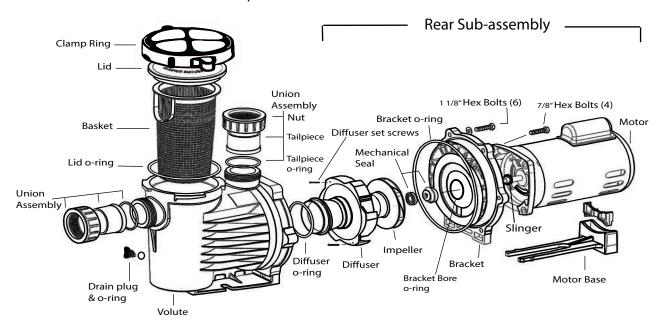
Disassembly and repair of the motor sub-assembly can be made as follows:
