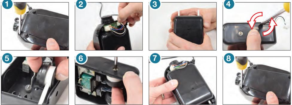
1. Unplug unit and remove four screws from bottom of main housing. Remove bottom of main housing to access internal housing.
