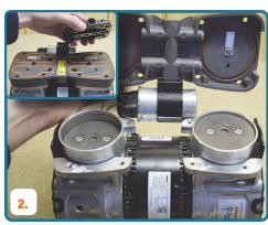
Mark the orientation of head plate(s) and remove. Mark the orientation of valve plate(s), remove valve plate(s). Clean valve plates with water based solvent, take care not to scratch valve seats.
