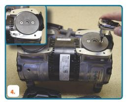
Remove screws from cup retainer plate with T15 Torx driver. Discard old cups and retainer screws.
