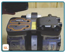
Reinstall head over valve plate(s) checking that orientation with ports is correct. Torque screws to 50 inch-pounds
