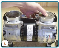
Press retainer plate with piston cup into cylinder all the way to the piston. The cylinder can be rotated to align the screw holes. Apply thread locking compound (Loctite<sup>®</sup> 222) to retainer screws, torque screws to 10-13 inch-pounds.
