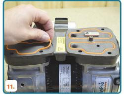
Remove old and install new head o-rings in the o-ring grooves on top of valve plate
