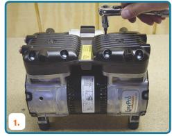
Remove screws from the head of compressor using T25 Torx driver, remove the head
