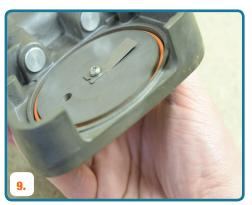
Inspect the leaf valves for damage or wear. NOTE: There is one intentionally "bent" leaf valve per set. If leaf valves need to be replaced, a complete leaf valve plate can be ordered. The screws holding the leaf valves are susceptible to breaking which makes individual leaf valve replacement very difficult.
