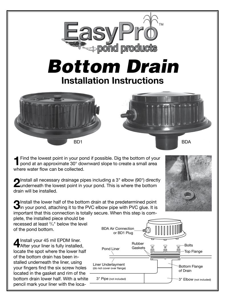
tion of the screw holes. Using an awl or punching tool, punch through the liner at the pencil markings being careful that the diameter of the punched hole is not wider than the diameter of the screw hole in the rim of the drain underneath the liner.
