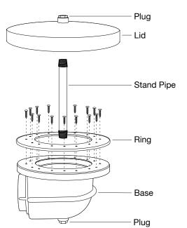
Drain base is installed under the liner, usually in the deepest part of the pond. Determine placement and excavate. Bottom drain and plumbing use a PVC 4" male adapter or reducing adapter to connect to PVC pipe (not included). Teflon tape threads of male adapter and tighten securely to prevent leaking.
