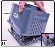
Repeat process on other side and reassemble housing, completely dried/cleaned filter and lid.
