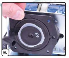
9. Line up new diaphragm to match how old one came off. Match up to notch on motor housing.
