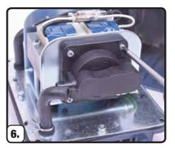
6. Remove the four screws from the plastic diaphragm housing with #2 Philips screw driver.
