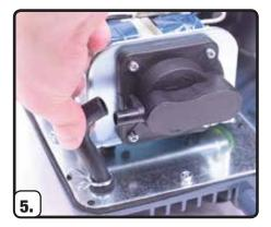
5. Repair one side at a time. Slide pinch clamp down the L-tube and remove top of L-tube from diaphragm outlet.
