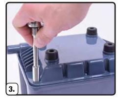
Turn unit upside down and remove four screws with either 8 mm nut driver/socket wrench (preferred) or #2 Phillips screwdriver.
