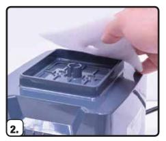
2. Clean filter pad with compressed air or with water. Must be completely dry before re-use.
