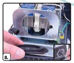
Unthread the 5.5 mm nut and remove the diaphragm from magnet. Note orientation of old diaphragm for proper installation of new one.
