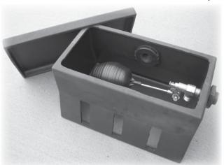
head fitting in the end that the auto fill mounts to. You will need to install the PVC bushing into the bulkhead fitting and then install the auto fill into the bushing. Use Teflon tape on all threads.
