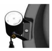
5. Install the 1/4" Flat Washer, 1/4" Lock Washer and 1/4" Nut against the underside of the float tab as shown in Figure 5. Tighten the nut until snug using the 7/16" Wrench.
