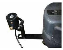
5. Install the 1/4" Flat Washer, 1/4" Lock Washer and 1/4" Nut as shown in Figure 10. Tighten the nut until snug using the 7/16" Wrench.
