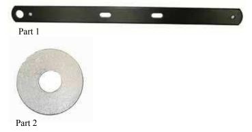
1. Turn the unit upside down. Loosen and remove the 3/8" nuts on the three 9" bolts that are closest to the motor unit. Place 2 Lower Float Brackets(Part #1) and one 3/8" washer(Part #2) on each of the 9" bolts over the bottom screen clips and replace the 3/8" nut.
